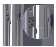
**Re-fasten** the plate to the post. Use alternate mounting holes if required. Test for proper function with hookbolt.
