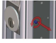
**Remove** the cylinder by unscrewing it counter-clockwise.
