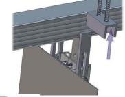
Loosen the hex bolts to adjust the height of the top stop.
