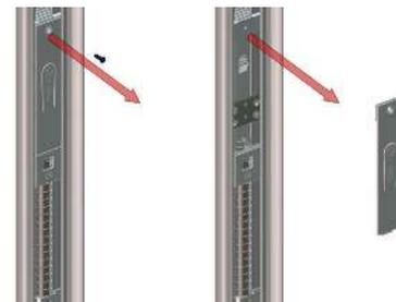
**Remove** the two screws in the lock plate.
