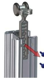
**Adjust** the height of the hanger. Use the indexing marks on the side of the post hanger as a guide (1/4" intervals).
