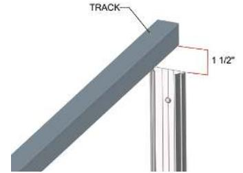
**Screw** to wall using 2" screws provided.
