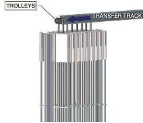
**Lift** the curtain and place the transfer track end-to-end with the installed track.
