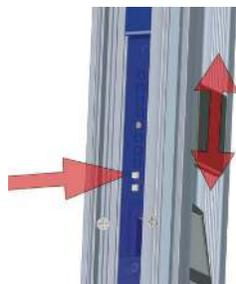
**Depress** the spring-loaded pins in the lock plate
