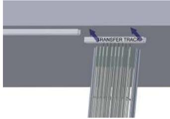
**Slide** the curtain section into the installed track.
