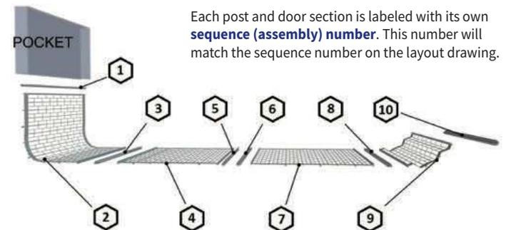
Each post and door section is labeled with its own **sequence (assembly) number**. This number will match the sequence number on the layout drawing.
