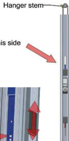
**The top lock rod** will always travel 1.5" from unlocked to locked, but the position is variable.
