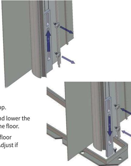
**Detach** trailing post from curtain (reverse directions in Step 5), and raise the bottom stop enough to pass over the V-stop.
