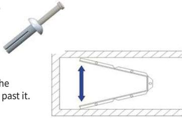
**Expand** the V-stop stop to ensure the trailing post won't be able to move past it.
