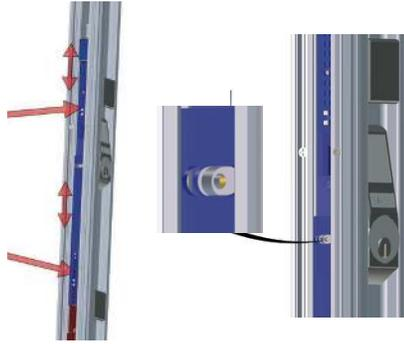
**Remove** the two screws in the lock plate.
