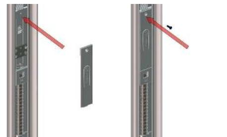
**Replace** the cover plate and retaining screw.
