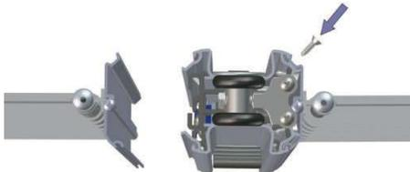
**Attach** by inserting the #6 self drilling screw in the screw channel. Place screws 2" from each end and spaced every 18".
