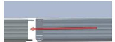
**Joint** must be tight with no gaps to ensure the trolleys do not catch and the door travels smoothly through the joint.
