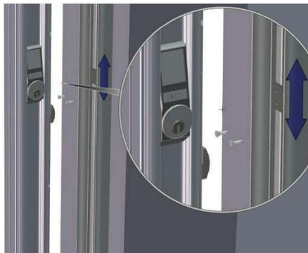
**Re-fasten** the plate to the post. Use alternate mounting holes if required. Test for proper function with hookbolt.
