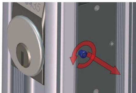
**Remove** the cylinder by unscrewing it counter-clockwise.
